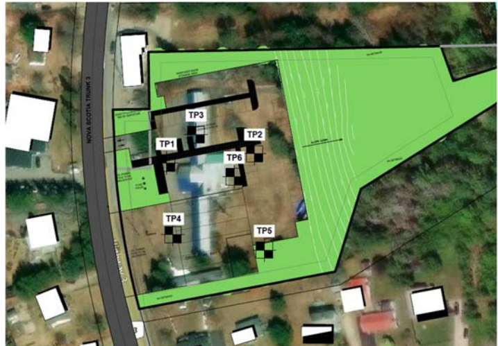
Figure A: Test Pit Locations
